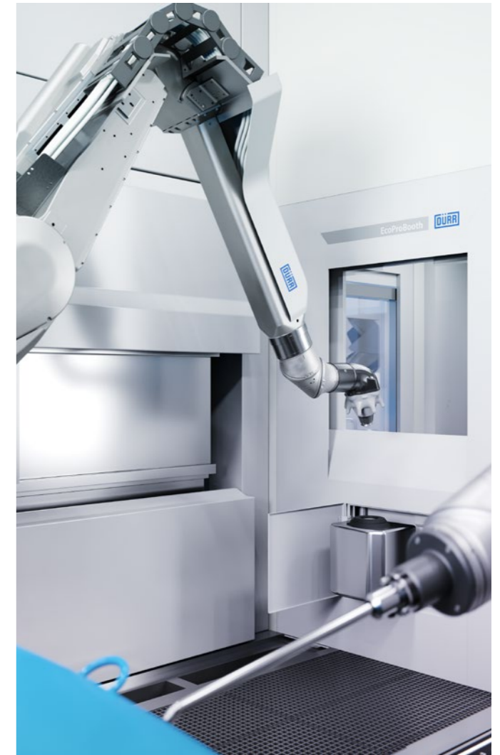
Maintenance without interruptions to production in the service cubicle.
