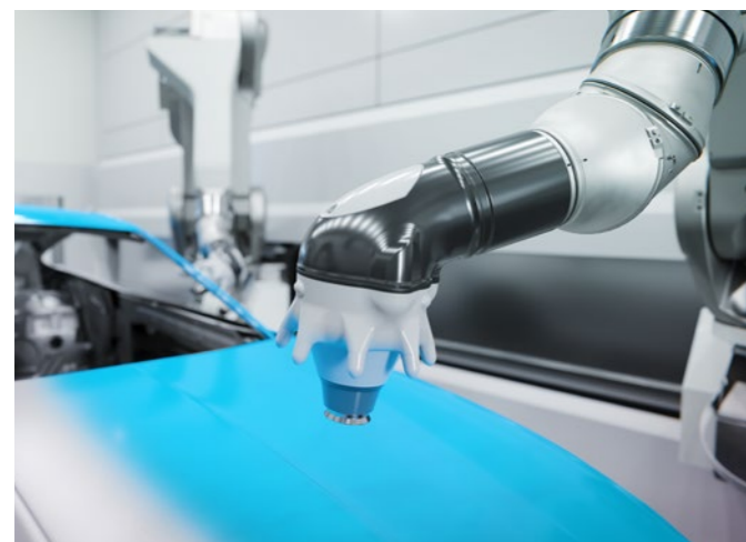
Interior and exterior painting in one booth with the EcoBell4 Pro Ux .
