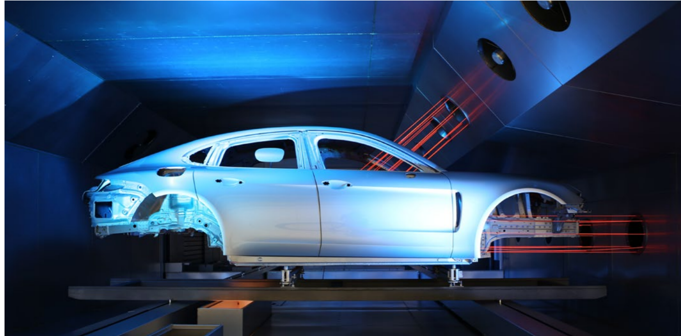
The bodies are transported crosswise, not lengthwise, through the oven.
