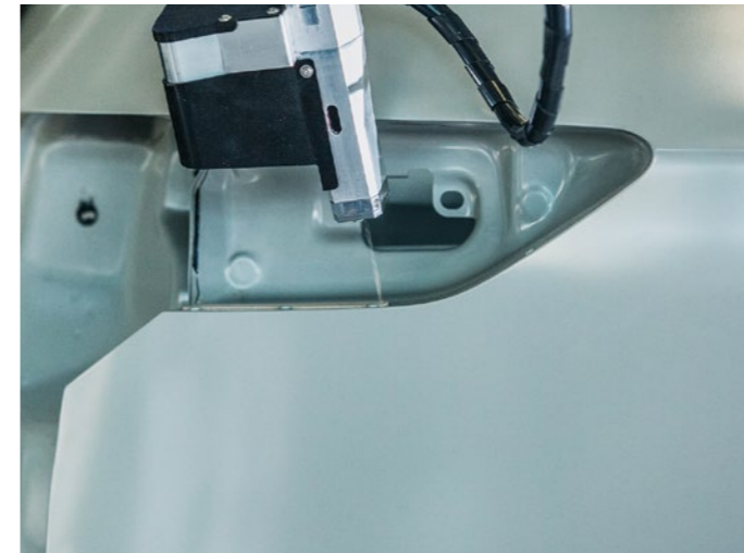
EcoSeaJet Pro also applies sealant to hard-to-reach areas automatically.
